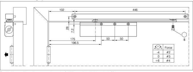
Provided the conditions allow, an opening angle of 130° is possible with this method of fixing. In most cases, however, a wall recess will have to be provided for the door closer.
