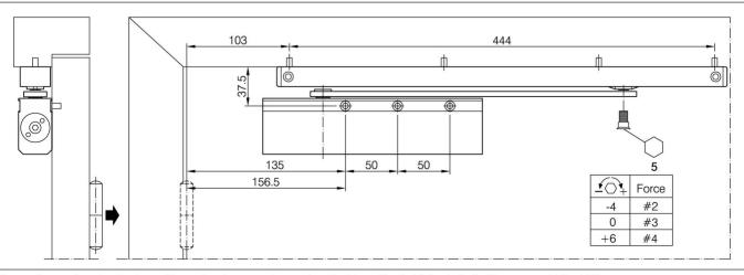
Depending on the structural conditions, the door opening angle with this method of fixing is limited to approx. 110°~130°. In order to avoid damage to the door or door closer, users are recommended to install a cushioned backstay or a door stop.
